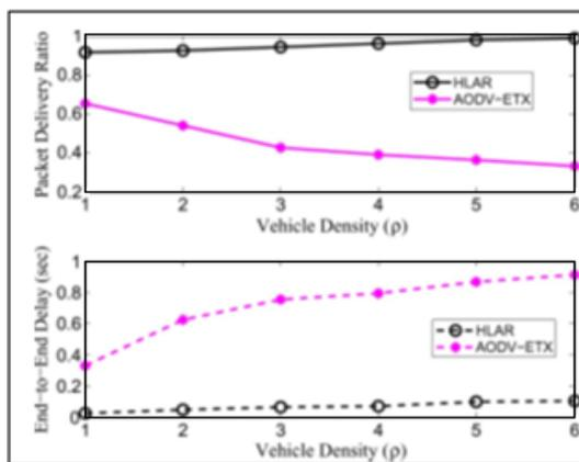
Figure 3 Packet delivery ratio and the end-to-end delay of the HLAR protocol compared to the AODV-ETX protocol as a function of the vehicle density ( $\rho$ ) in [nodes per 2000 m<sup>2</sup>].
